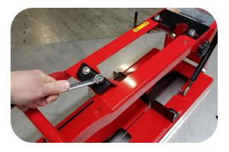
**3.** Unhook retention chain and raise head of Portaband Pro jig. Next, disconnect the ball joint that connects the gas shock to the top of the jig.
