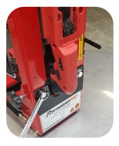
**11.** Using the included 3/32" hex key and an 11/32" wrench, reinstall the yellow trigger arm as shown below.
