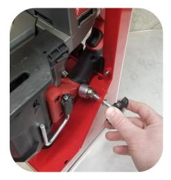
**9.** Pivot the base of the jig up to meet the bandsaw. Check blade alignment within the slot in the base. Using a 3/4" wrench, slightly loosen the three bolts at the base of the jig so that it can be adjusted for blade alignment.
