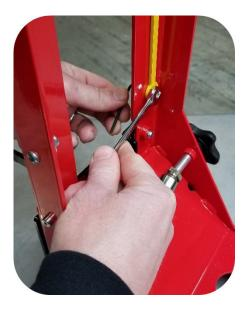
**5.** Using a 9/16" wrench, loosen the two bolts that retain rear adjuster plate, so that the adjuster can easily slide side to side.
