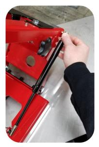
4. Using the included 3/32" hex key, and an 11/32" wrench, remove the yellow trigger arm and hardware from under the top of the jig. Save for reinstallation in step 11.
