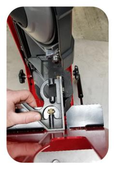
**10.** Using a 1/2" wrench, tighten the two bolts holding front handle bracket. Tighten adjuster plate using a 9/16" wrench.
