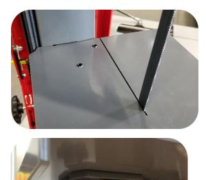
**3.** Slide the table over the material guide and into the small slot at the back of the saw. Clamp the washer and hand knob to the bottom of the guide.
